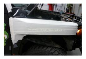
**4.** Tape template to mudguard making sure it is lined up with top of mudguard (bonnet opening) and rear of mudguard (door opening).
