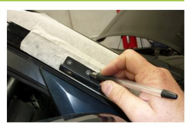
12. Install snorkel body to vehicle using M8 Nylock Nuts and body washers provided and attach to pillar bracket using M6 bolts provided.
