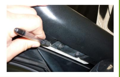
**11.** Hold bracket in position previously marked on pillar and mark mounting holes.
