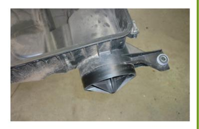
**15.** Refit air box for vehicle, attach to rubber joiner and attach with hose clamp provided.
