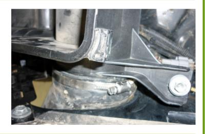
**16.** Check all hose connections and air box for potential leaks and seal as required.
