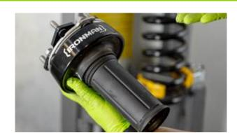
**18.** Using a 15mm socket and supplied M10 nuts, reinstall the strut assembly into the vehicle.
