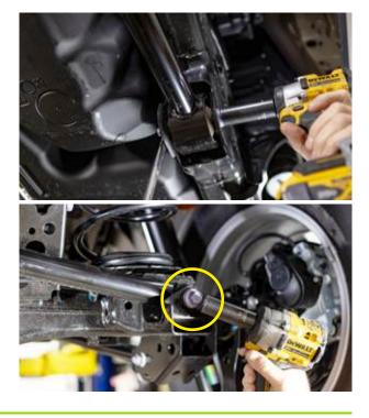
**26.** Using a 17mm socket, disconnect the sway bar end link from the chassis.
