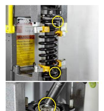
**13.** Carefully remove the spring isolator from the strut top, taking care not to remove the dust boot.
