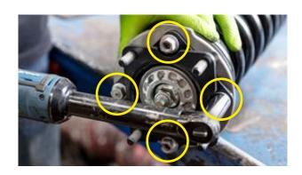
12. Position the strut assembly in an applicable spring compressor, ensuring the lower bushing hole is right angled to you.
