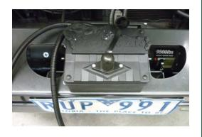
5. Connect three colour coded cables to the corresponding poles on winch motor.
