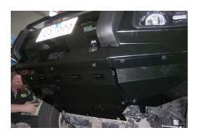
16. Trim mud guard liners level with protection plates and secure with cable tie.
