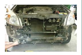
3. Place U-Bolts in position around chassis from inside out, in front of radiator.
