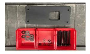
4. Start on the right-hand side of the vehicle. Locate the front and middle body bolts. Unbolt and keep bolts aside to re-install later.
