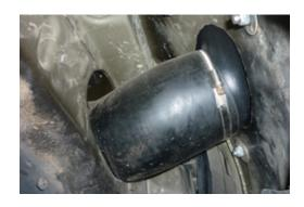
**14.** Remove foam seal from air box intake.
