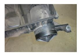
**15.** Refit air box for vehicle, attach to rubber joiner and attach with hose clamp provided.
