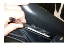
**11.** Hold bracket in position previously marked on pillar and mark mounting holes.
