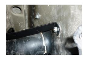
**13.** Attach rubber joiner to snorkel with outlet towards front of hole in engine bay and secure with hose clamp provided.
