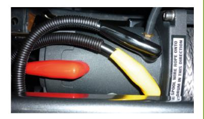
**5.** Connect the thin black earth wire and negative battery cable to the earth connection on the opposite side of winch motor.
