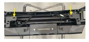
**35.** Feed N#12 Right and Left N#11 nut plates into position.
