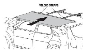
Carefully and tightly roll the awning material back towards the main body, reversing the set up procedure and secure in place with Velcro straps.
